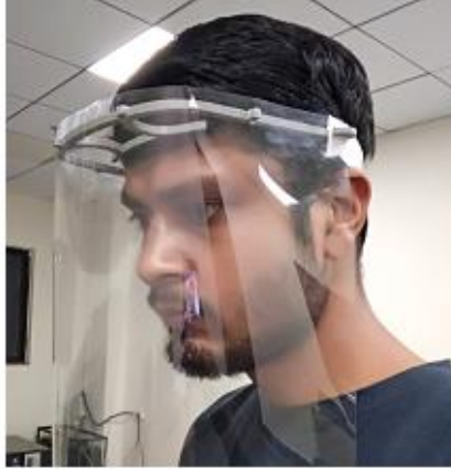
Newly developed face shield prototype to be manufactured using laser cutting process
