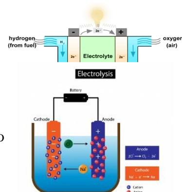
**Electrolysis** The research area is metal powder production via electrolysis. This research will significantly increase energy efficiency and reduce greenhouse gas emissions for metal production. When two half reactions are combined that do not lead to spontaneous production of energy, electric potential must be applied for the overall redox reaction to proceed. In the example electrolytic cell above, molten NaCl is converted into chlorine gas and sodium metal via electrolysis.
